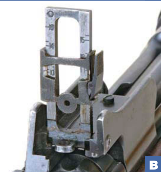
(A) Earlier, the Model 1905 rear sight on the Model 1903 Springfield was a masterpiece of craftsmanship, which is why it was discontinued in the wartime emergency of 1941/1942. Raised, it offered a small peep. Lying flat, its battle zero was set for 500 meters. (B) The peep rear sight of the British-designed US Model 1917 was a fine battle sight, but lacked windage adjustment. (C) Duke considers the US Model 1903A3 to have a fine rear sight because it is a windage adjustable peep type. (D) The M1 Garand rear sight was arguably the best sight ever issued on a battle rifle. This one is the WWII "locking bar" version. (E) The M1 Garand (below) was loaded by means of an 8-round "en bloc" loader, most commonly called a "clip."
